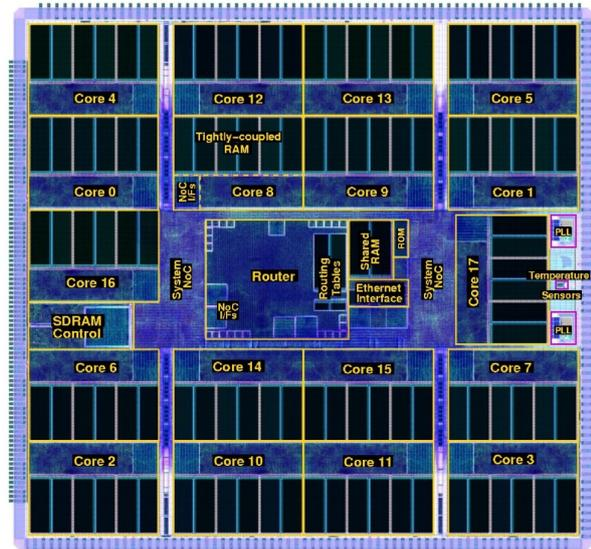
Globally Asynchronous Locally Synchronous (GALS) chip:
